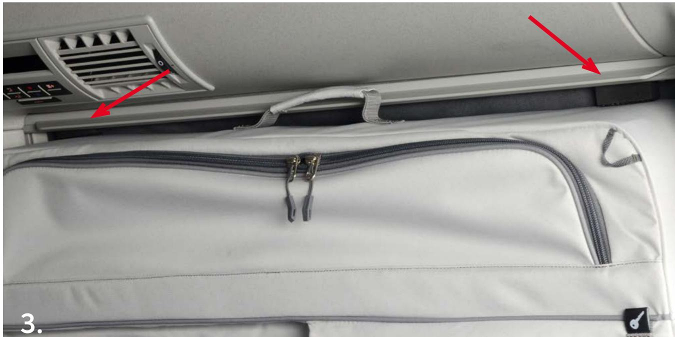
Thread the rear panel of the packing bags behind the sun blind (pic. 2) then push the bags into the window (pic. 3).
