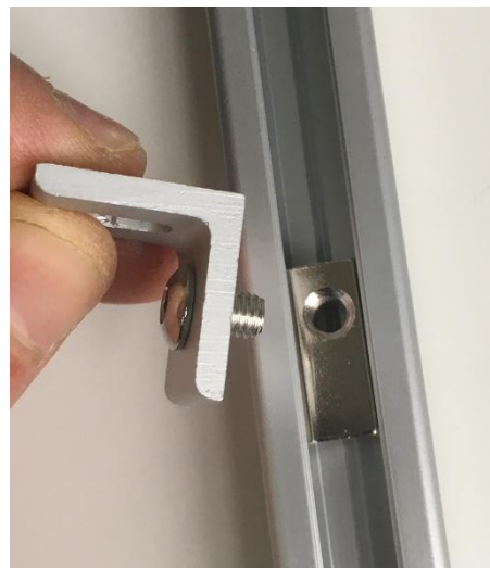
Figure 3. Attach brackets (C) using round head bolts (E).
