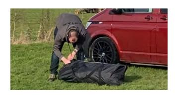
11. Roll awning towards you, squeezing out air as you go, once rolled tie with strap and pop into carry bag
